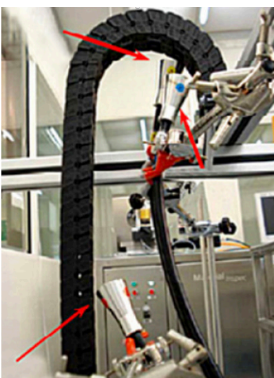
Figure 1: Optical Particle Counters in Critical Cable Chain Areas
